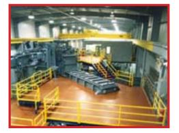
Masteralloy VIM systems are generally in the range of 1-10 tons and are characterized by their ability to pour many multiples of small diameter ingots configured on a mold car or turntable. Masteralloy ingots are commonly as small as 73 mm ( $2^{7}/_{8}$ ") and as large as 254 mm (10") in diameter and generally about 1.2m (48") tall. Consarc Masteralloy VIM systems commonly incorporate the following features:
