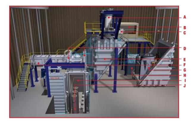
Vacuum Induction Melting (VIM) is the melting of metal via electromagnetic induction under vacuum. An induction furnace containing a refractory lined crucible surrounded by an induction coil is located inside a vacuum chamber. The induction furnace is connected to an AC power source at a frequency precisely correlating to the furnace size and material being melted.
